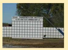
These photos show a breakaway sign in action. Breakaway signs make collisions with signs safe for the vehicle occupants.
