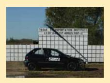
"Breakaway signs" include supports that, when struck by a vehicle, separate from the base and are knocked ahead of or up and over the errant vehicle, as well as supports that "yield" or allow the vehicle to run over them. Note that compliance with this standard is required by January 2013 for all nonbreakaway sign supports within the clear zone of roads posted at 50 mph or greater.
